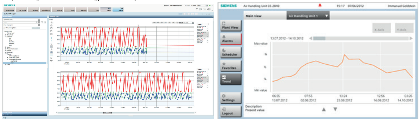
Trend viewer on the management platform Desigo CC and on the touch panels PXM40/PXM50
